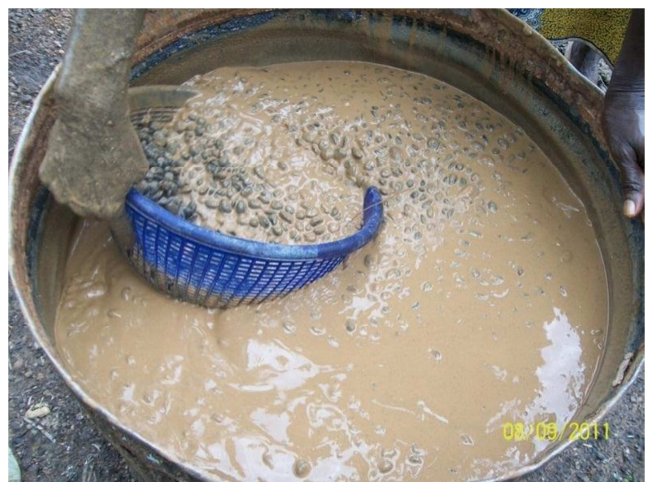
Figure 3. Clay-water bath method of separating palm kernels.
