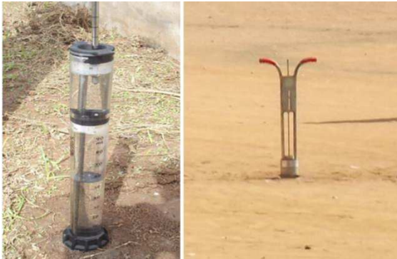
Figure 3. Field set up for MiniDisk Infiltrimeter (right) and set-up of Turf-Tec Infiltrimeter (left) Source: Field Survey 2015, 2018.
