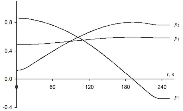
Figure 3. Changing the components of unit vector  $p$  in time under optimal control.
