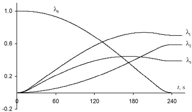
Figure 2. Changing the components of orientation quaternion  $\Lambda(t)$  during optimal reorientation.
