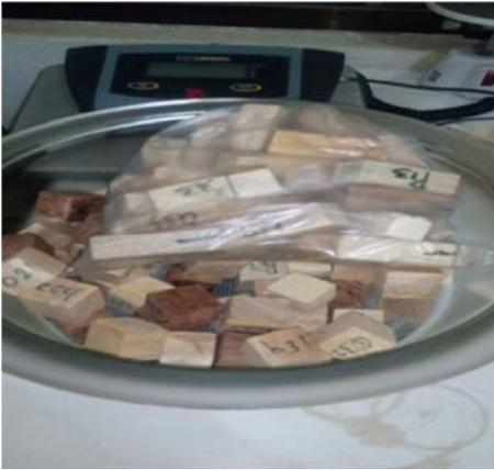
Figure 2. Modified wood samples inside dessicator.
