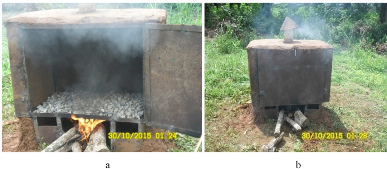
Figure 3. a. Constructed Smoking Cabinet Showing Drying Chamber; b. Constructed Smoking Cabinet Showing the External Features.
