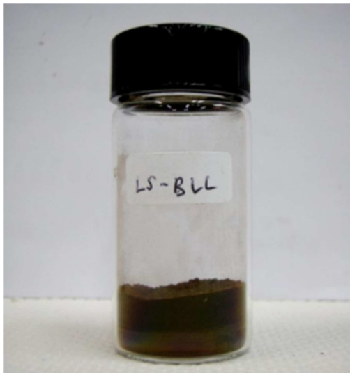
Figure 2. Lignosulfonate produced after sulfonation process.
