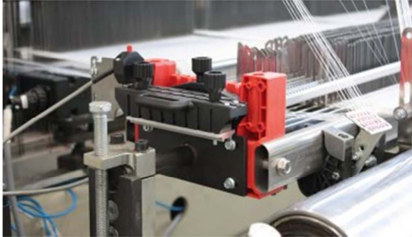
Figure 16. The Falling of the Dropper Cutting the Flow of the Laser Beam [11].
