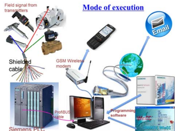
Figure 7. Architecture of plant automation.
