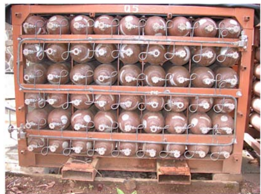
Figure 9. Helium Quad with interconnecting manifold.
