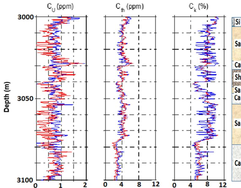
Fig. 4. Results of tests with synthetic data for a hypothetical well. Red curves indicate synthetic data before optimization while blue curves represent results obtained after the optimization. The column on the right indicates the lithology (Si – Silt; Sa – sandstone; Ca – Calcutite; Sh – Shale)
