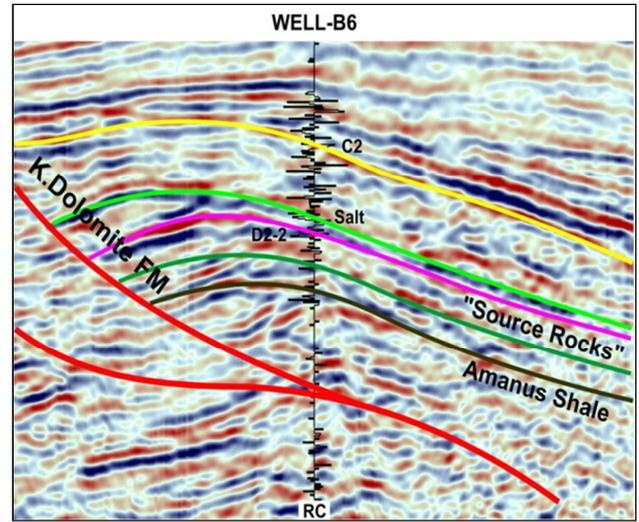
Figure 6. Reflectivity coefficient (RC) calculated from well logs indicate tight correlation of well data with the seismic data (see CD position on Figure 2).
