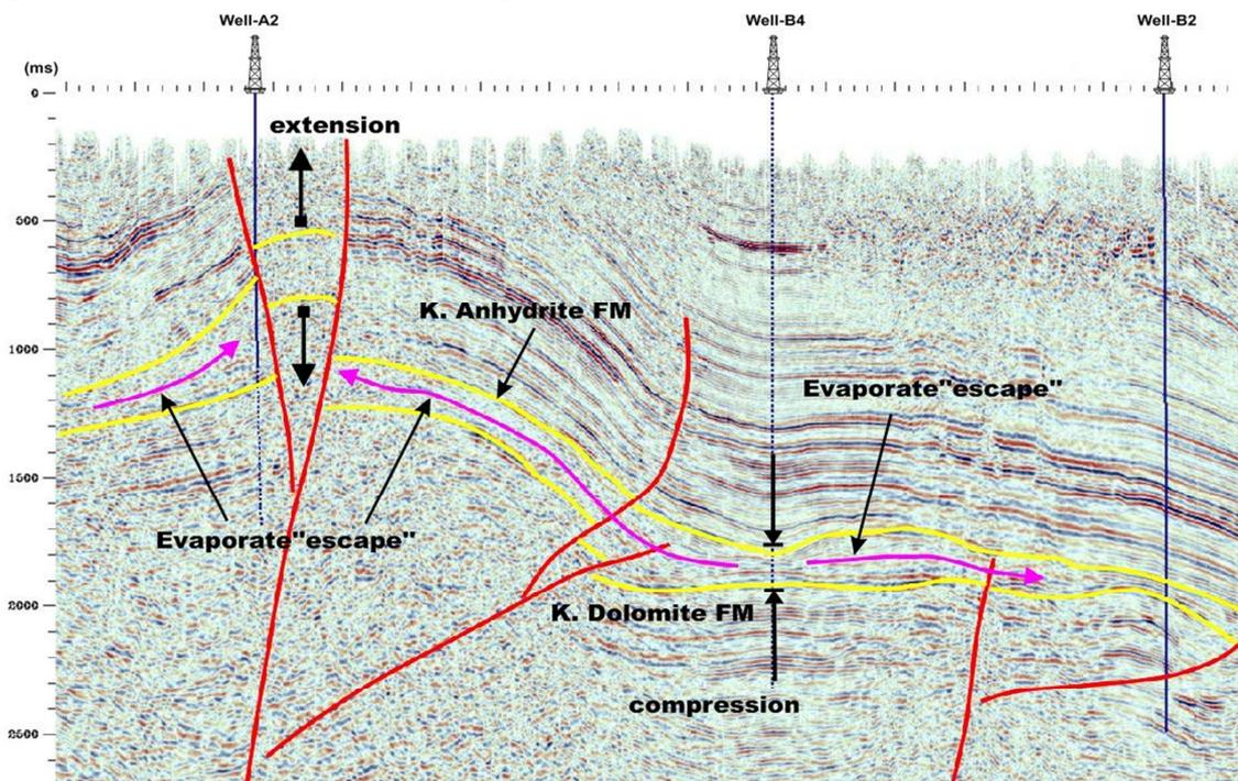
**Figure 8.** Escape of evaporates as a consequence of the compressional tectonic which also created positive flower structure in area of A2 well and highly influenced the thickness of evaporates.
