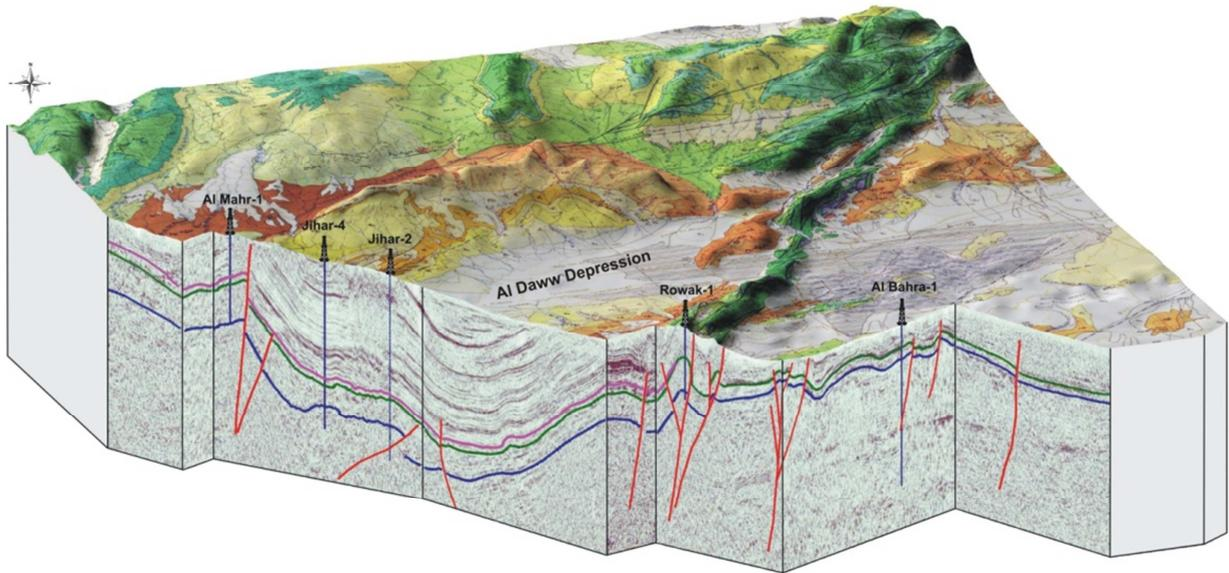
Figure 4. Block diagram of Hayan Block. Violet - top D2-2 (main source rock, Kurrachine Dolomite FM), green - bottom source rock, blue - top Markada FM..
