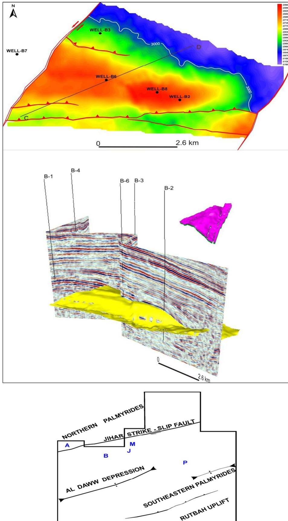
**Figure 2.** Structure map on the top of the mature source rocks of the Kurrachine Dolomite Formation (“B” oil/gas field, position above); Seismic section with extracted top of the source rock Unit (yellow) and 3D shape of the source rock body (magenta). -Volume of Unit =  $1.4 \times 10^9 \text{ m}^3$ ; mass of hydrocarbons generated HCG =  $1.27 \times 10^{10} \text{ kgHC}$ ; Oil generated =  $0.8 \times 10^8 \text{ bbl}$  or  $12.7 \times 10^9 \text{ m}^3$  of oil equivalent (Vulama, 2011).
