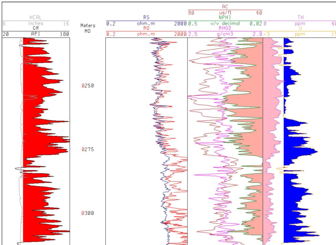
Figure 7. Composite log of the Kurrachine Dolomite Formation, "B"-6 well. Note high Uranium (U) content of total GR.
