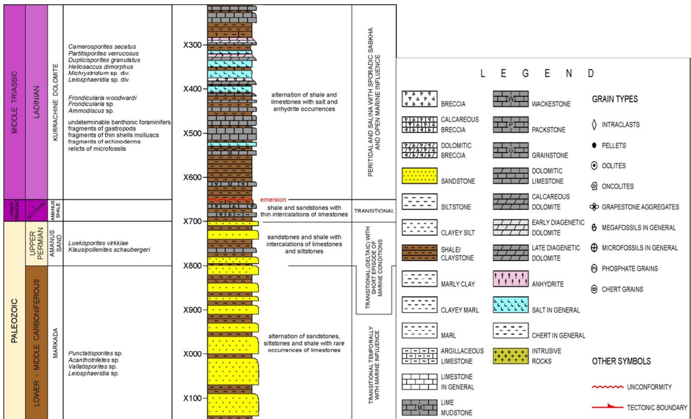
Figure 5. Typical Paleozoic and Triassic successions of Hayan Block with local lithology, depositional environment and biostratigraphical assemblage (modified after V. Veseli, personal communication).
