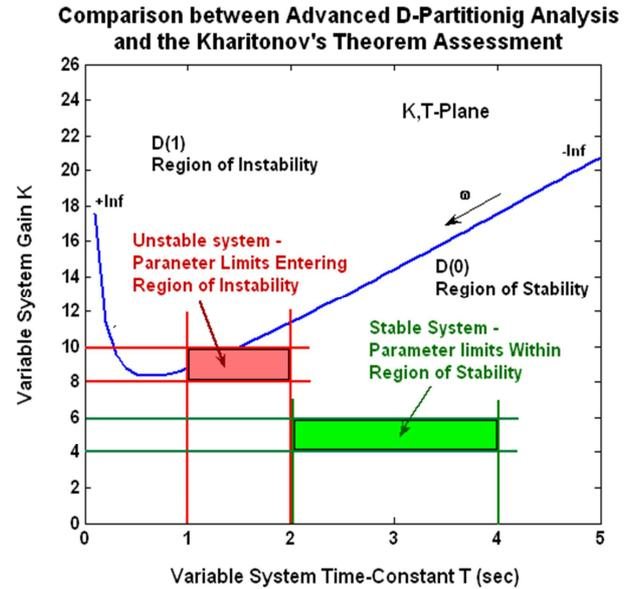
Figure 10. Comparison between the Advanced D-Partitioning Analysis and the Kharitonov's Theorem Assessment in Terms of Two Simultaneously Variable Parameters.
