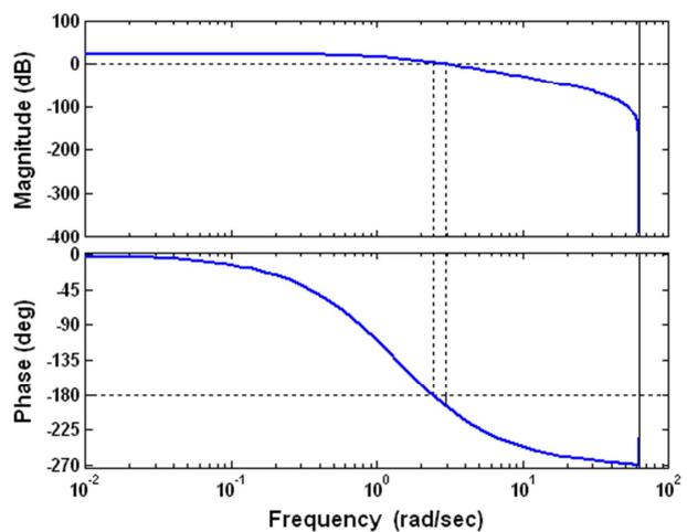
**Figure 9.** System's Instability Result from the Advanced D-Partitioning in Case of Two Variable Parameters, confirmed by the Bode Stability Criterion in the Discrete-Time Domain.
