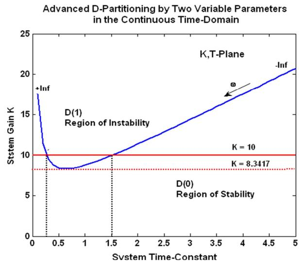
Figure 6. Advanced D-Partitioning by Two Variable Parameters in the Continuous-Time domain.
