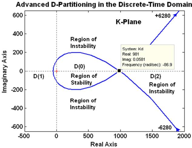
Figure 3. Advanced D-Partitioning in Terms of the Variable Gain Factor  $K$  in the Discrete-Time Domain.
