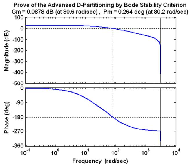
Figure 5. Confirmation of the Result from the Advanced D-Partitioning with the Aid of the Bode Stability Criterion in the Discrete-Time Domain.
