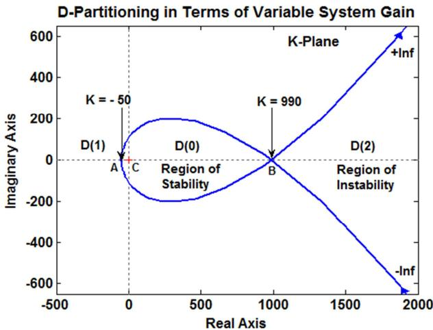
Figure 1. D-Partitioning Facilitated by the “dpartition” m-code.
