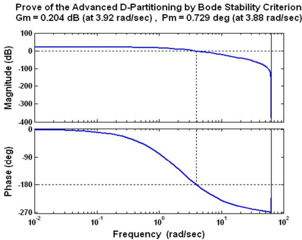
**Figure 7.** System's Marginal Result from the Advanced D-Partitioning in Case of Two Variable Parameters, confirmed by the Bode Stability Criterion in the Discrete-Time Domain.
