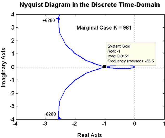
Figure 4. Confirmation of the Result from the Advanced D-Partitioning with the Aid of the Nyquist Stability Criterion in the Discrete-Time domain.
