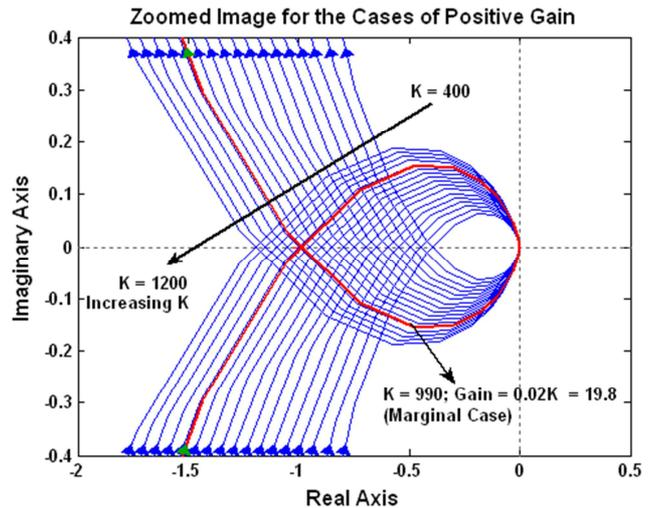
Figure 2. Zoomed Image of the Marginal Gain, Confirmed with the Aid of the Nyquist Stability Criterion.
