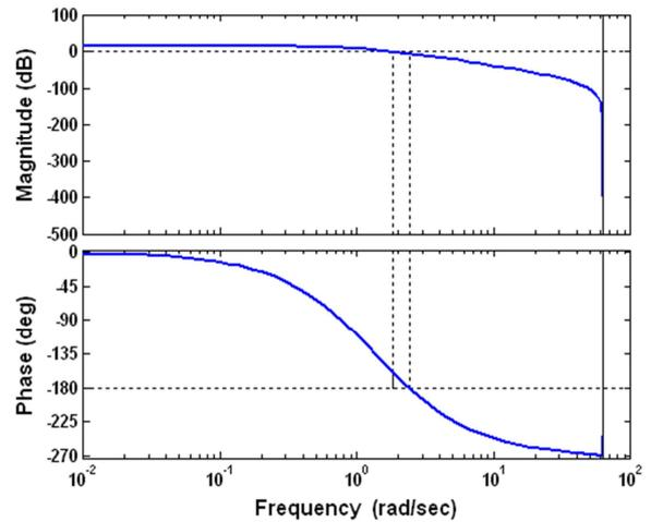
**Figure 8.** System's Stability Result from the Advanced D-Partitioning in Case of Two Variable Parameters, confirmed by the Bode Stability Criterion in the Discrete-Time Domain.
