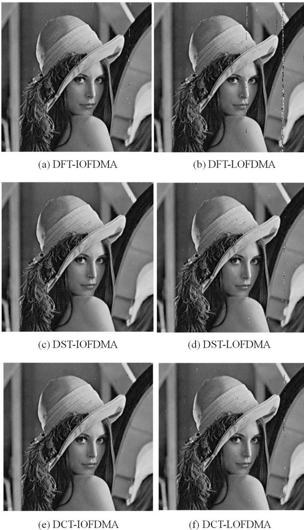
Figure 8. Image for different OFDMA Systems at SNR = 20 dB and QPSK.
