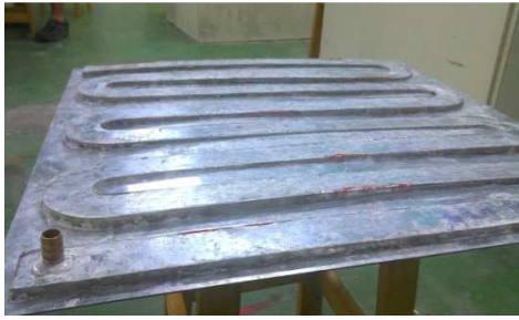
Fig 7. Photo of the heat exchange device of piping tablet.
