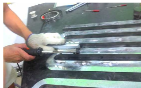
Fig 6. Welding process of the heat exchange device of piping tablet.
