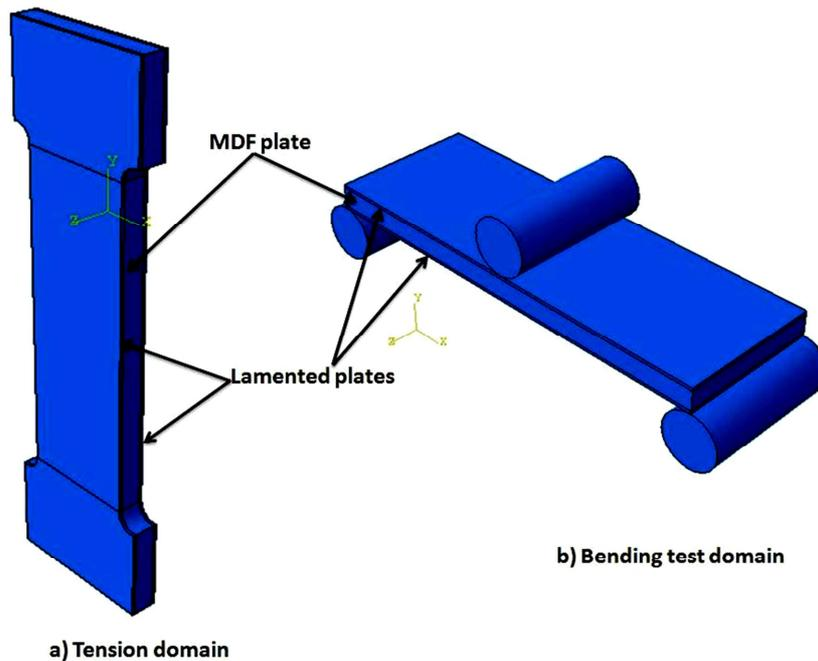
Fig. 1. Finite element domain a) Tension b) Bending
