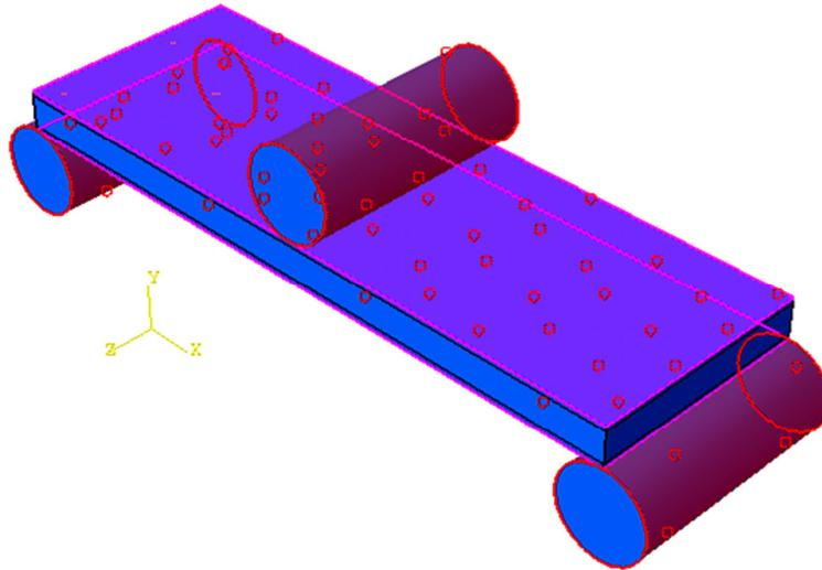
Fig. 5. Interaction between supporting and load roller
