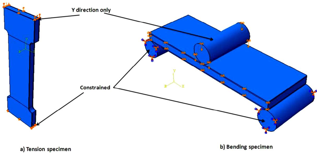
Fig. 4. Boundary condition a) tension test b) bending test
