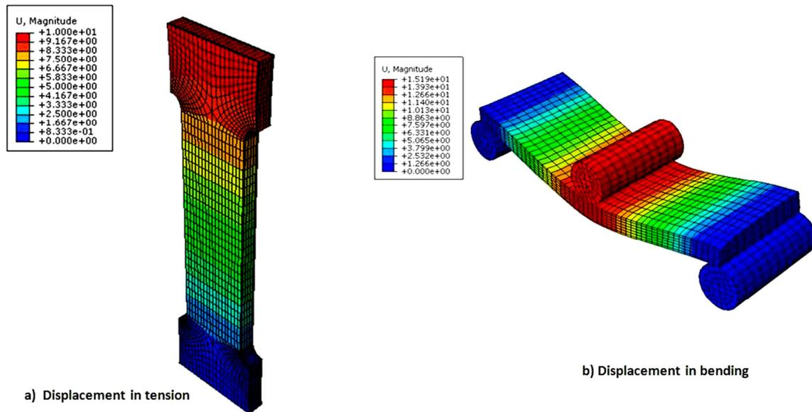
Fig. 11. Finite element displacement prediction in a) tension test b) bending test
