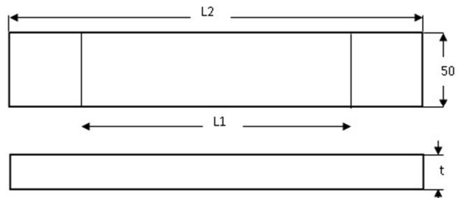
Fig. 7. Stander three point bending test specimen (dimension in mm)
