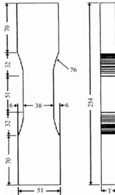
Fig. 6. Stander tensile test specimens (dimension in mm)
