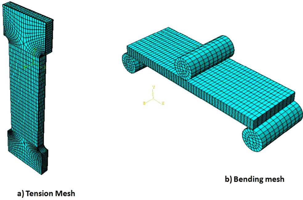
Fig. 2. Mesh domain for a) tension specimen b) bending specimen
