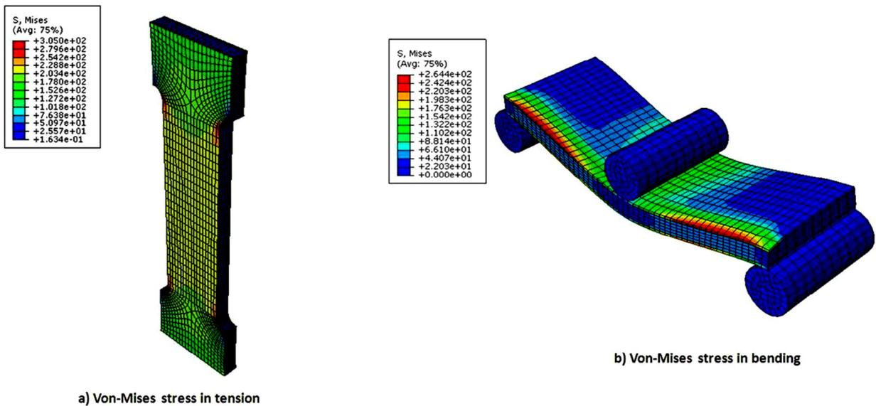
Fig. 10. Von-mises stresses prediction in a) tension test b) bending test
