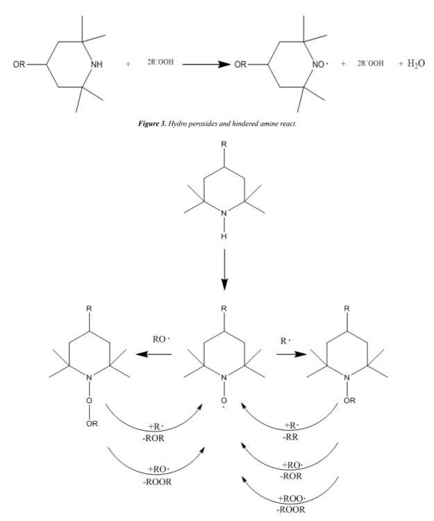
Figure 4. Radical-trapping mechanism of hindered amine.
