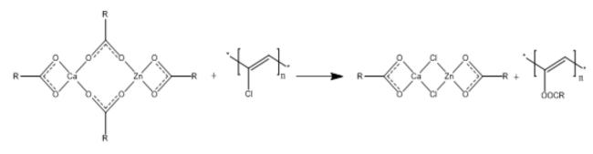
Figure 2. PVC and calcium zinc composite stabilizer react.
