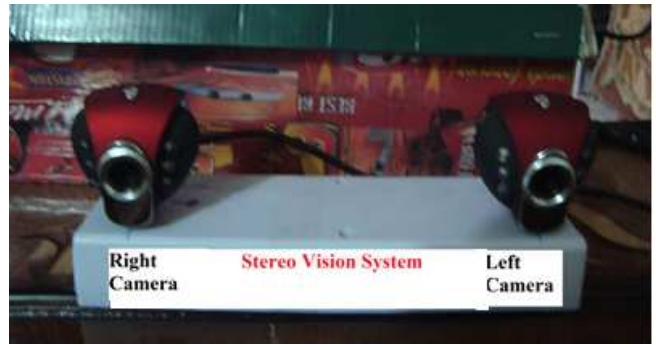
Figure 11. The implemented stereo vision system.
