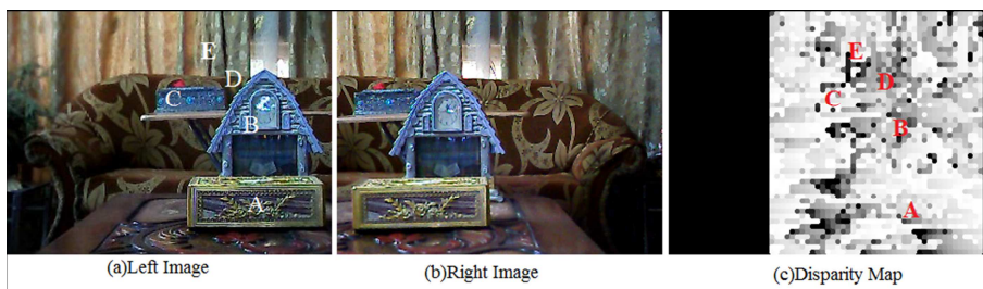
Figure 12. Stereo images captured by the practical stereo cameras and the disparity map by selecting points at different depths.
