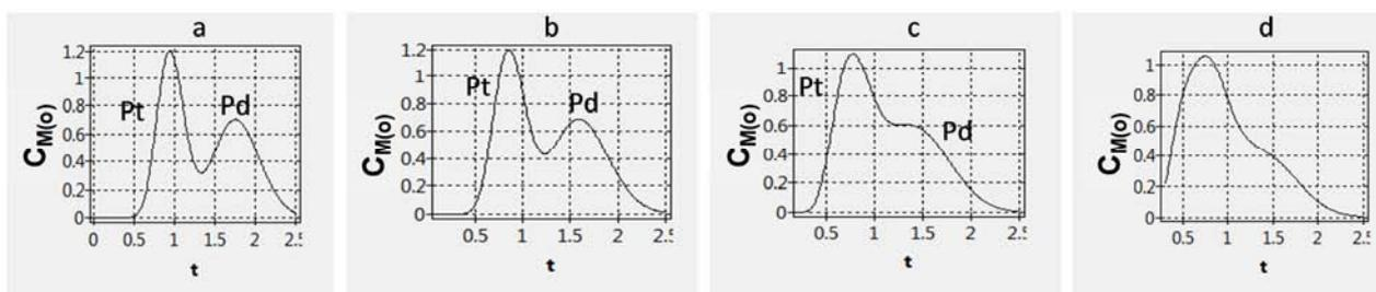
**Figure 1.** Calculated chromatograms (organic phase) of the palladium and platinum mixtures separation ( $K_{D(Pd)} = 0.28$ ,  $K_{D(Pt)} = 0.52$ ) for the first cycle of counter-current process for different sample loading time ( $t_s$ : 0.01 (a), 0.1 (b), 0.2 (c), 0.3 (d) at  $N = 100$ ,  $t_x = 0.5$ ,  $t_y = 0.4$ ).
