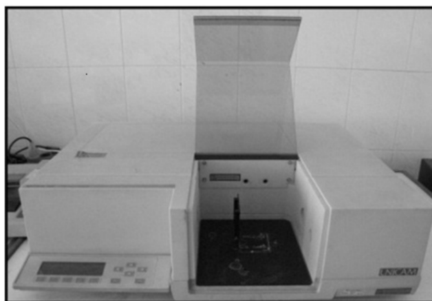
Figure 12. FTIR device used to detect bisindolylmethane surface groups.
