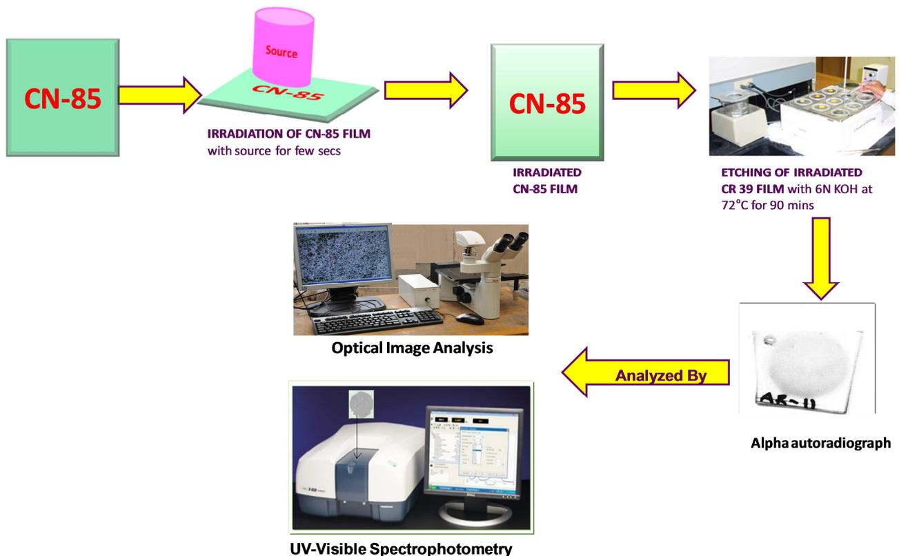
Figure 1. Schematic of alpha imaging and analyses carried out in the study.
