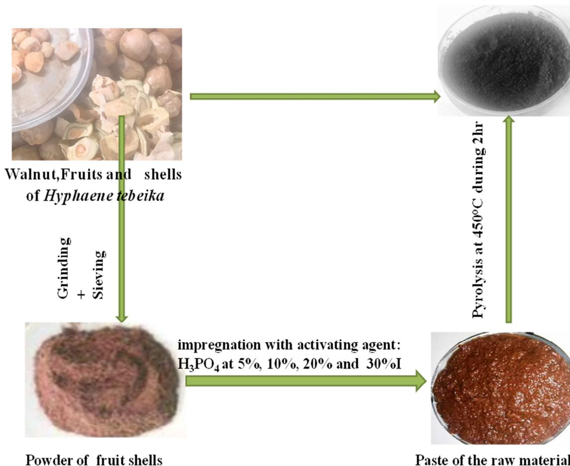
Figure 1. Steps on the preparation of activated carbon.
