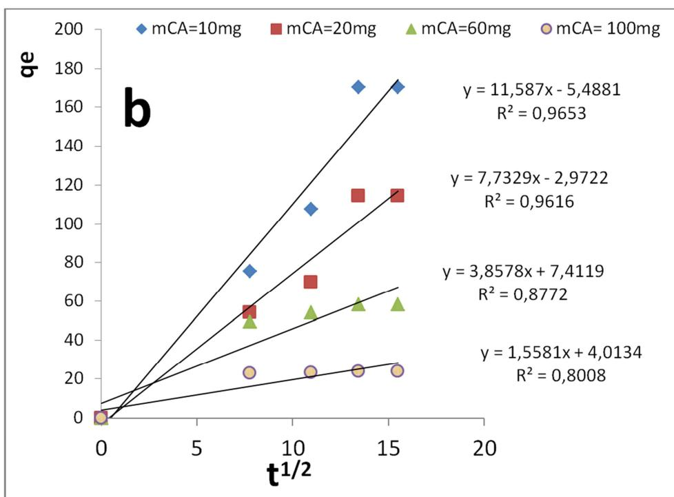
Figure 8. (a) plots of PCBs congeners uptake against square root of contact time, and (b) Linear regression curves of intra particle diffusion on AC10.
