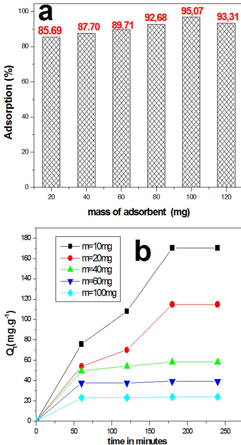
Figure 4. Adsorbent mass effect on adsorption of PCBs congeners (a) and Contact time effect for different masses of AC10 ( $C_i = 25\text{PPM}$ ,  $\text{pH} = 6.48$ ,  $T = 30^\circ\text{C}$ ) (b).
