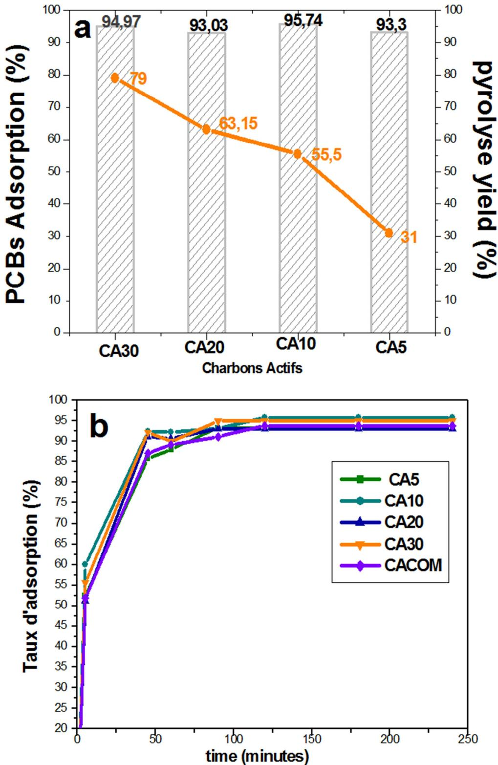
**Figure 3.** (a) Comparison of pyrolysis rate and adsorption capacity of prepared activated carbons; (b) Determination of Equilibrium time for adsorption of PCBs in aqueous solution. ( $C_i=25\text{PPM}$ ;  $\text{pH}=6.5$ ;  $m_{AC}= 100\text{mg}$ ; at room temperature)
