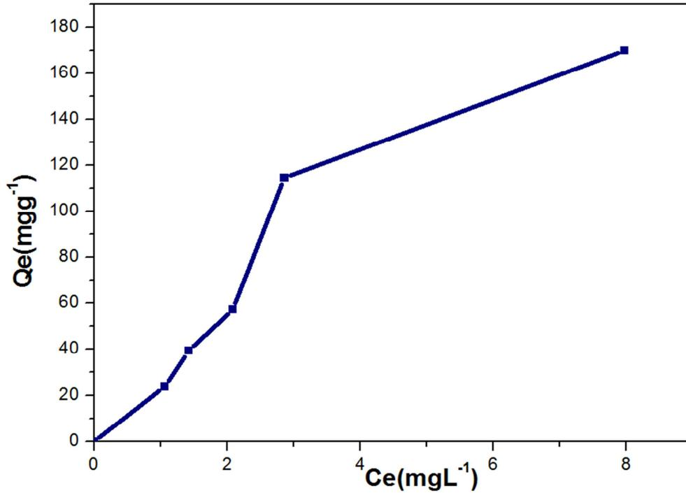
Figure 6. Equilibrium Adsorption isotherm of PCBs on AC10 (mCA= 100mg, pH= 6.5 at room temperature).
