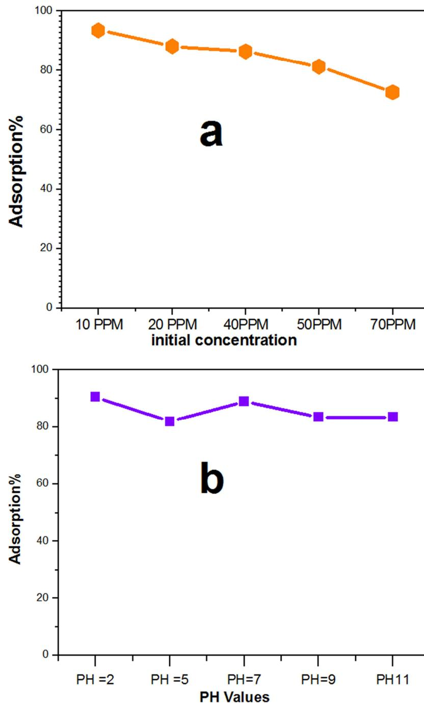
**Figure 5.** Effect of initial concentration on PCBs adsorption ( $m_{AC}=100\text{mg}$ ,  $pH=6.48$ ) (a) and Effect of PH on PCBs adsorption ( $m_{CA}=100\text{mg}$ ,  $C_i=25\text{PPM}$ , at room temperature,) (b).
