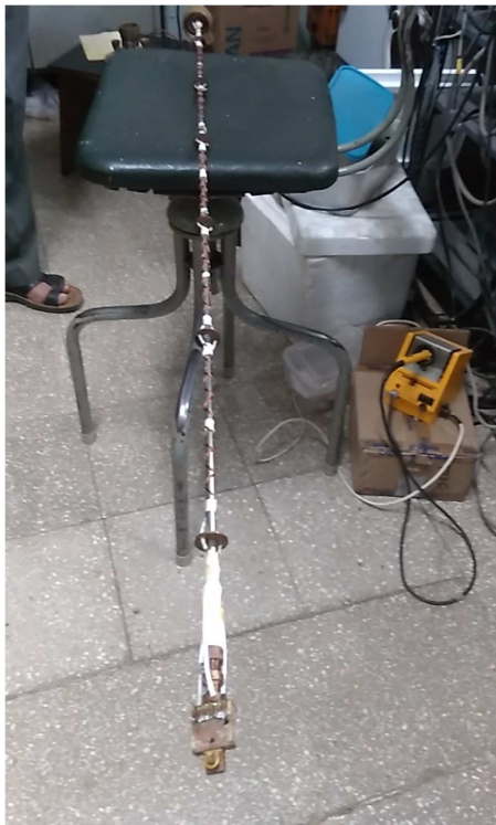
Figure 4. In-house fabricated Variable Temperature Insert (VTI).
