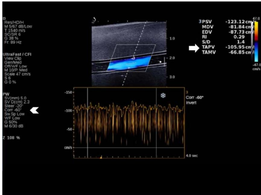
Figure 2. UFCD velocity estimation of a continuous parabolic flow moving at 106 cm/s. In the top, the UFCD map with a 20° CD-box steering angle and a 10° probe tilting angle. In the bottom, the spectrum derived from the retrospective processing of the ultrafast.
