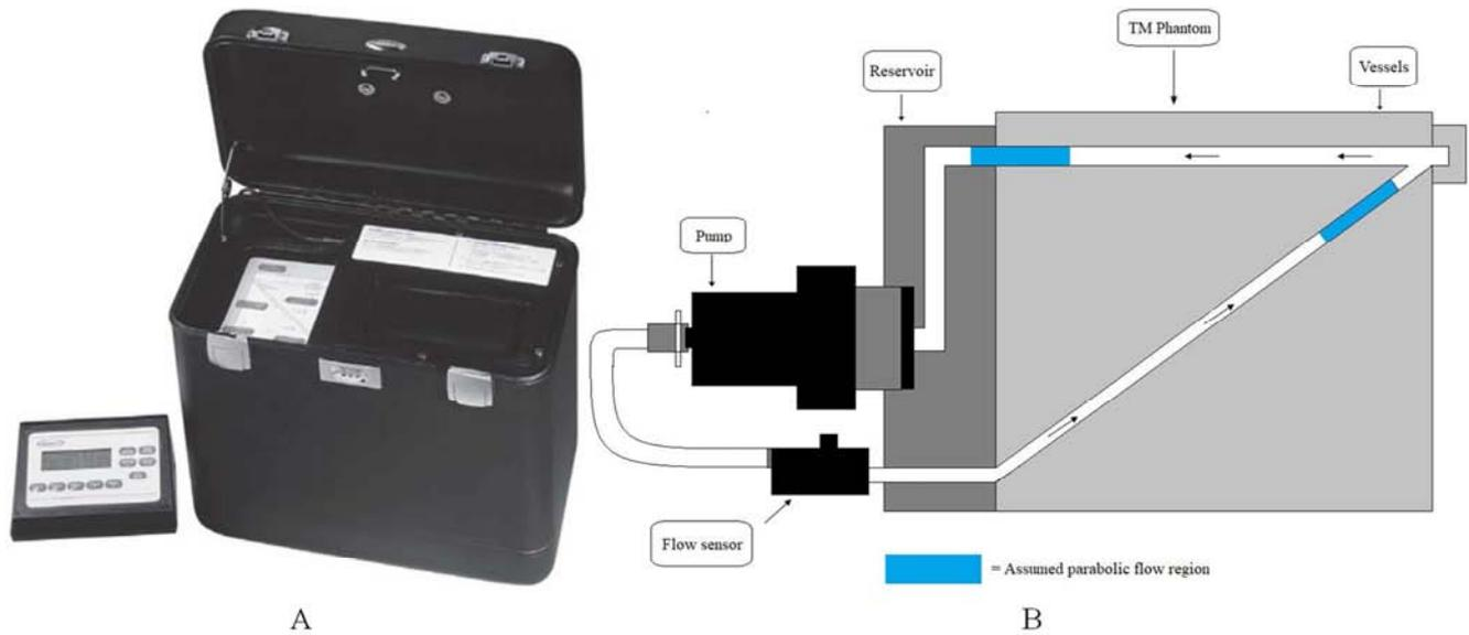
**Figure 1.** The Gammex 1425A used for the acquisitions (1a) and its scheme (1b). 1b shows the zones where the flow is assumed to be parabolic by the manufacturer.
