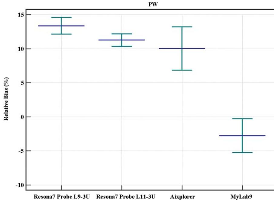
**Figure 5.** Parameters assessing the performance of different systems and techniques in the velocity estimation, based on 10 repeated measurements at three peak velocities for parabolic flow (35, 70, and 106 cm/s).
