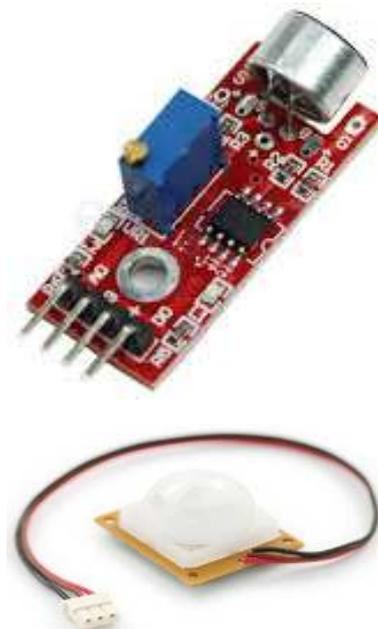
Fig. 2.2. (a) Voice Sensor (b) PIR Motion Sensor.
