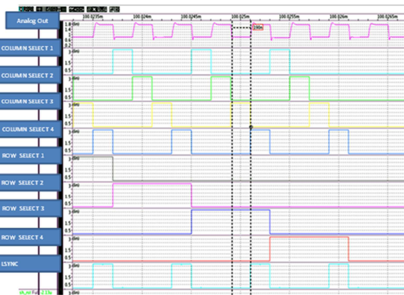
Fig. 7. ROIC Analog Output and other signals for consecutive high/low input signals.
