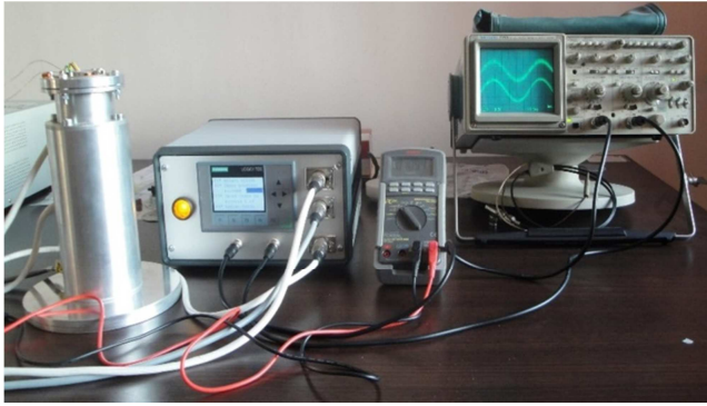
Figure 6. A setup for measuring voltage on a hybrid core tooth winding.
