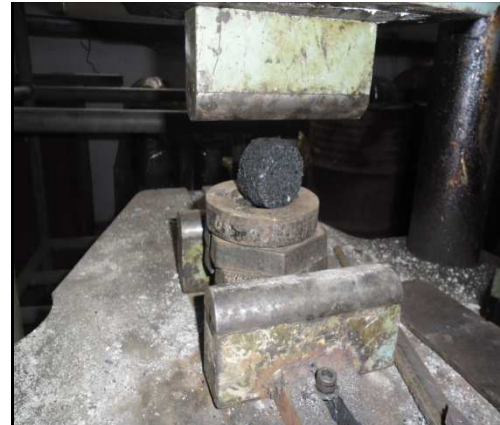
Figure 6. Cleft Failure Conditon Test
