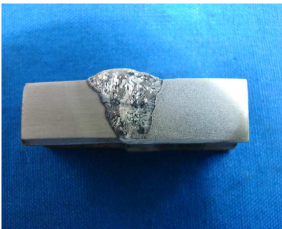
Figure 9a. Macro examination T92+ASS 347H.
