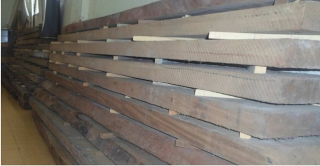
Figure 2. Pericopsis elata wood in natural drying in the laboratory.
