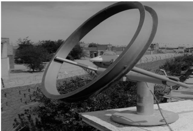
Figure 1. Pyranometer for measuring the diffuse radiation data in site of the test cell.
