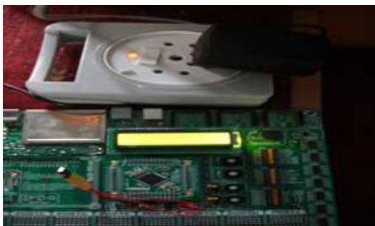
Figure 6. Interfacing of temperature Sensor to Embedded PLC
