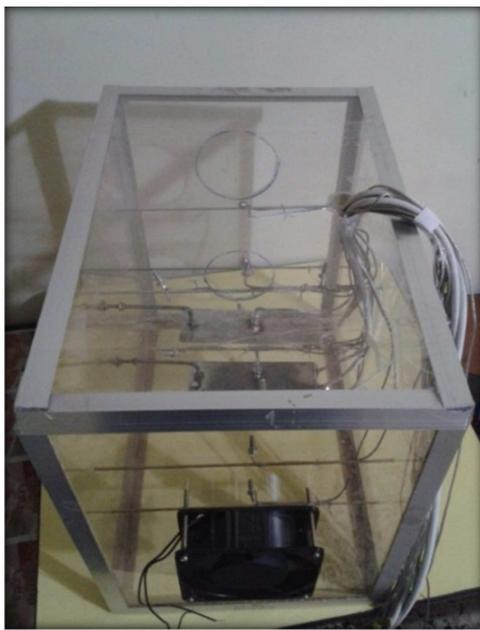
Figure (4). Thermocouples distribution on grid inside test section.
