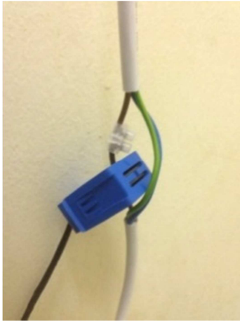
Figure 3. Setup of the current sensor with live wire.
