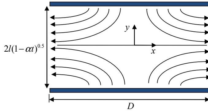
Figure 1. Flow configuration and coordinate system.
