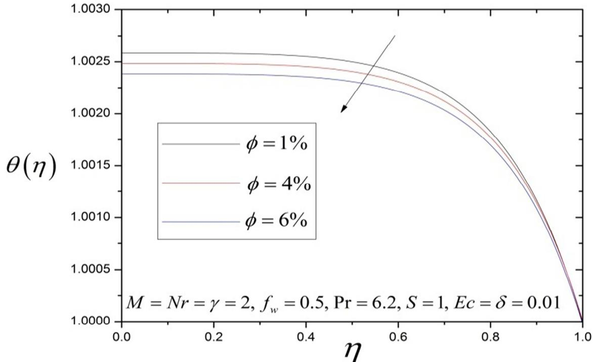
Figure 10. Variation in temperature  $\theta(\eta)$  due to several values of  $\Phi$ .
