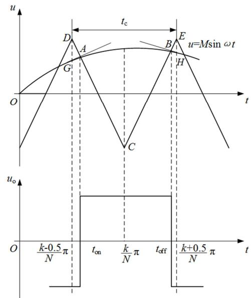
Figure 4. Double tangent sampling method.
