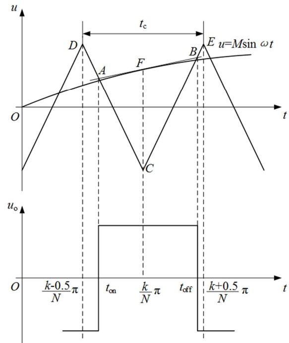
Figure 2. Tangent sampling method.
