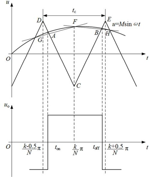
Figure 3. Secant sampling method.
