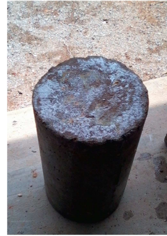
Figure 11. Cylindrical specimen attack by \text{MgSO}_4 .
