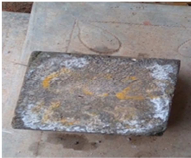
Figure 10. Cube specimen attack by \text{MgSO}_4 .
