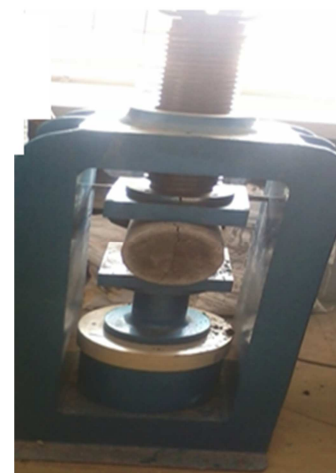
Figure 9. Split Tensile Strength test on concrete cylinder.
