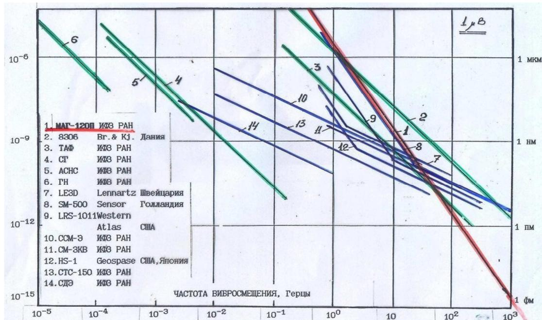
Figure 2. Comparative characteristics of some seismic devices.
