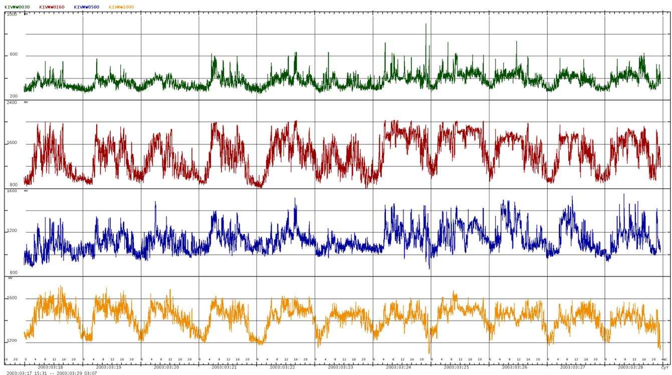
Figure 5. Record acoustic noise in the frequency bands (from top to bottom): 30, 160 500 and 1000 Hz.
