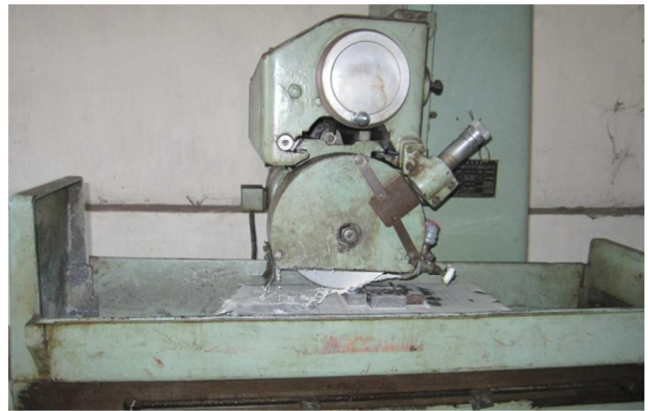
Figure 1. M7120A surface grinder.
