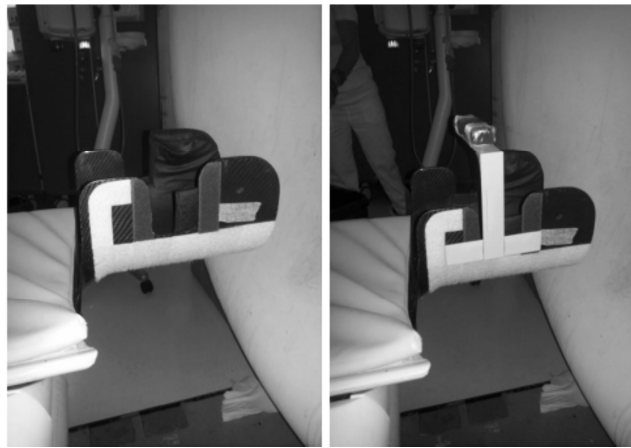
Figure 9. Developed height adjustable system for shielding set-up [18].
