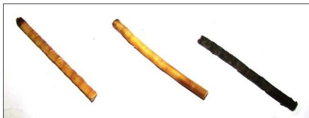
Figure 1. Cores taken at the beam head (right), in its middle part (central) and its foot, near the ground (left).
