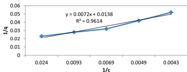
**Figure 3.** Langmuir Isotherm for MG Adsorption.
