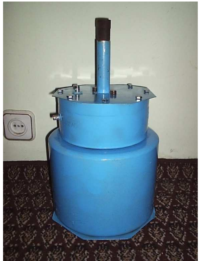
Fig. 5. The photograph of the Faraday's cage.
