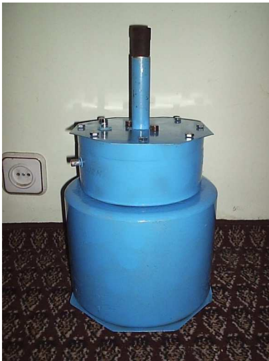
Fig. 21. The photograph of the Faraday cage.
